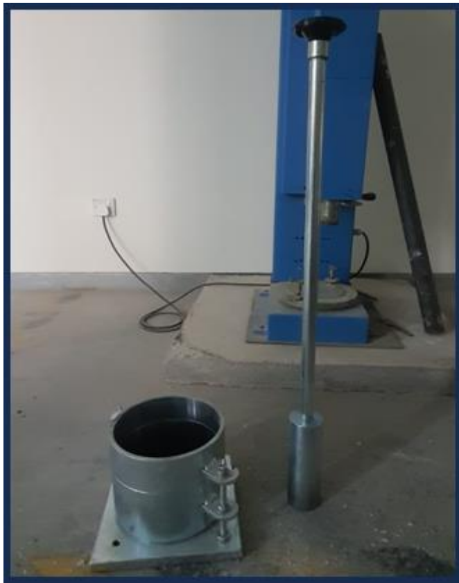
Figure 4.7. Iron rod and heavy metal cylinder for crushing samples
